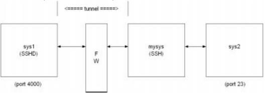
For example, a user wants to use mysys to create a tunnel between sys1:4000 and sys2:23, so that TELNET sessions that originate on sys1:4000 get tunneled to sys2 through the firewall. On mysys, issue the command:
